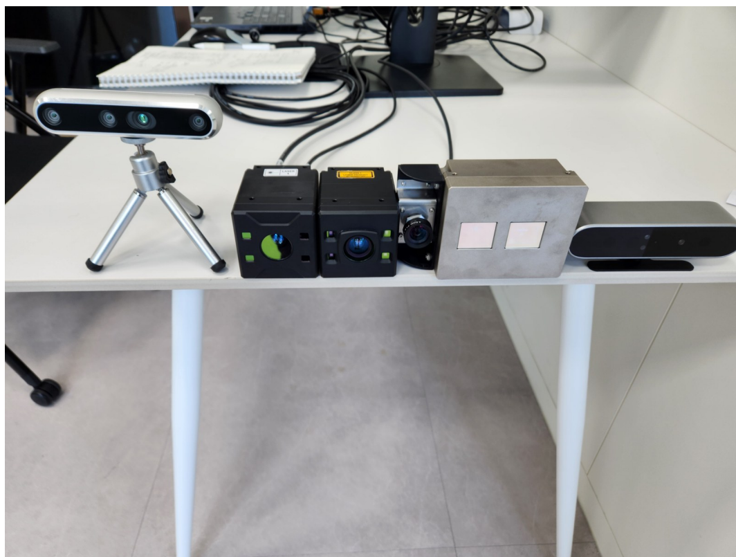
Figure 3. The five commercial 3D sensors put through validation: three ToF, one structured-light, one active-stereo
