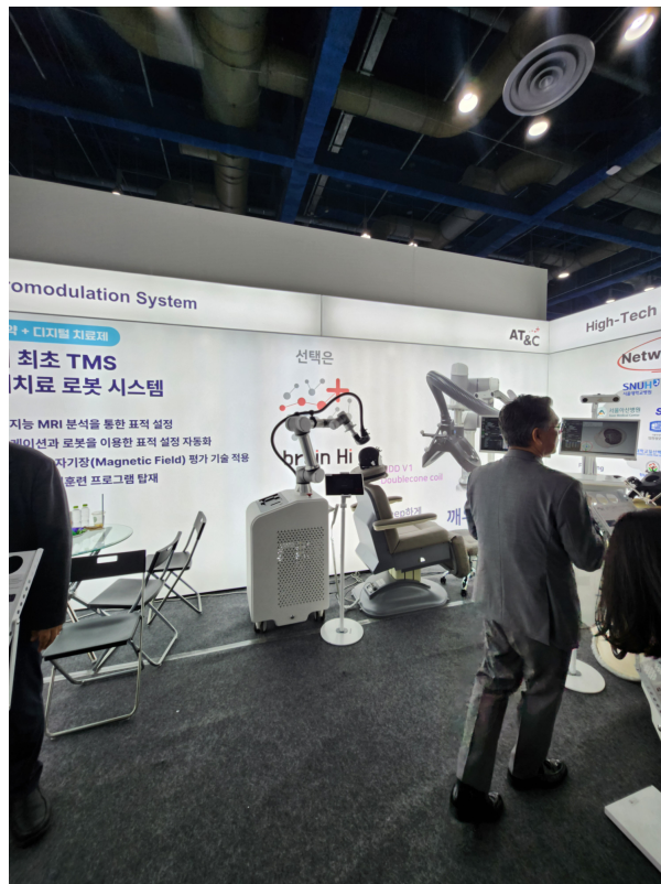
Figure 1. Demonstration of the TMS coil-navigation robot system on an exhibition stand: robot arm, treatment chair, coil, and navigation displays in one setup.
